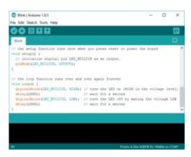
Programming the A-Star 328PB from the Arduino IDE.
